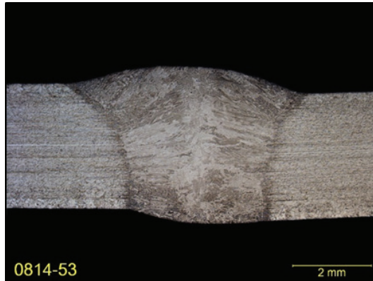
Figure 4. Macrograph for the PQR weldment (right) produced in 5 in. schedule 10 Type 304 stainless steel pipe using 308L EWI DeepTIG wire
