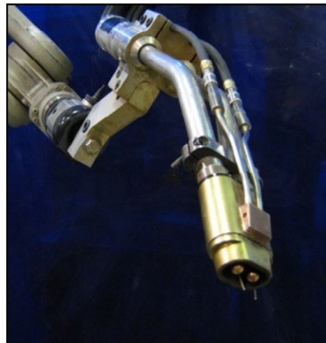
Figure 2: Tandem GMAW torch mounted on a 6-axis robot
