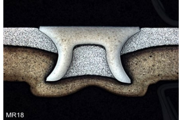
Figure 6: Mechanical joint between Al-6111 and an Mg-AZ-91 alloy
