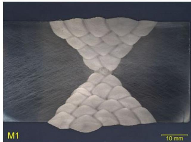
**Figure 1: Multi-pass GMAW weld made on 1.5-in thick magnesium**
