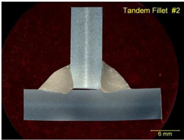
**Figure 2: T-GMAW fillet welds made on 1/4-in thick 6061 Aluminum at a travel speed of 60-ipm**
