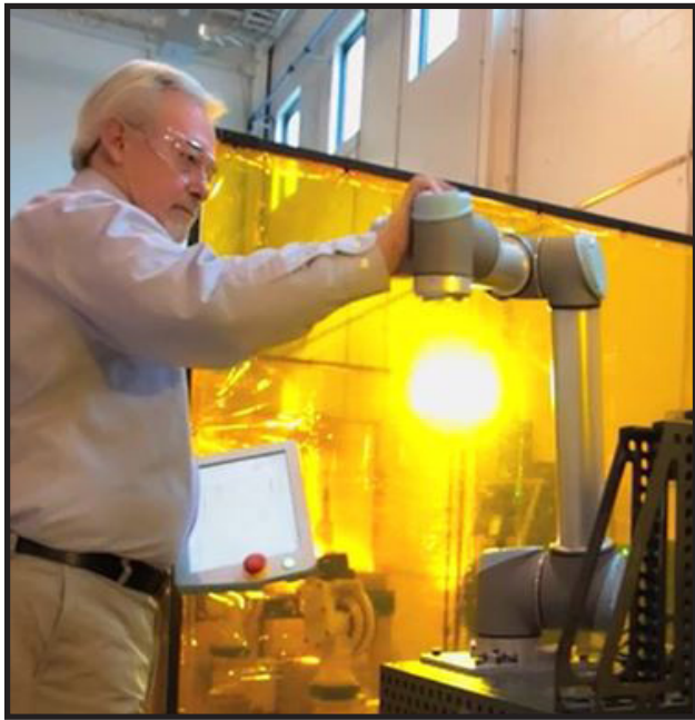
Figure 4: Cobot with drag-to-teach capability
