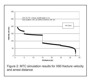
The MTC model was then used to optimize the design of pipe segment arrangements for a mockup full-scale burst test using high-strength pipeline steel. The MTC simulation results confirmed the experimental observation that different pipe arrangements result in different arrest toughness and arrest distance for pipes of the same grade. As a result, the MTC model can be used for running fracture control in modern pipeline design and vintage pipeline integrity assessment.
