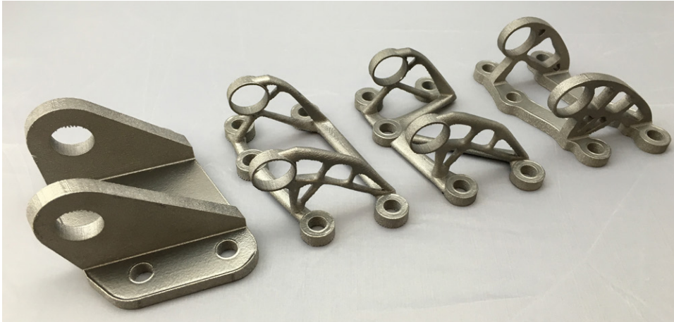
Figure 1: Part redesign cycle for a topology-optimized aerospace bracket.
