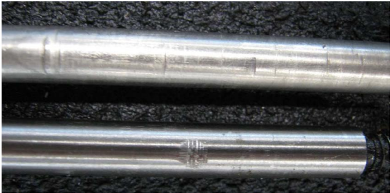
Figure 12. Photograph of Scarred Center Post used to Align the Belleville Washers in the Fast Follow-Up Head (Scarred surface prevented the head from providing follow-up action.)
