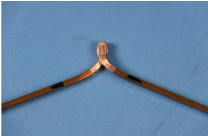
Figure 4. As-Welded Parallel-Wire Joint Geometry
