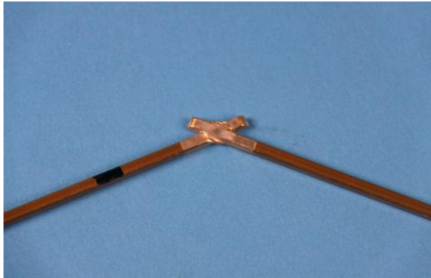
Figure 3. As-Welded Cross-Wire Joint Geometry
