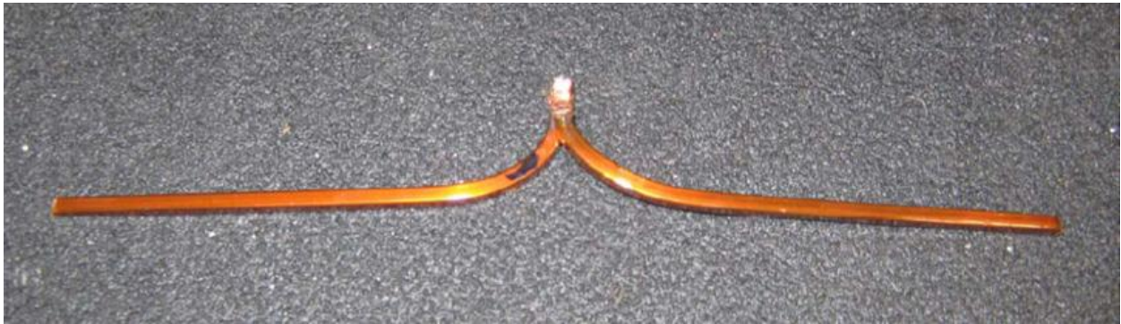
Figure 11. Weld Sample Prepared for Tensile Testing (Parallel-Wire Geometry Shown)
