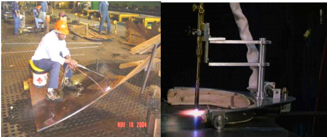
Figure 2: A conventional line heating process (left) and an automatic line heating device developed by EWI for Navy ManTech project (right)
