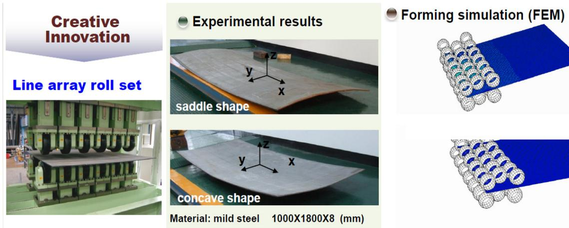
Figure 3: Line Array Roller Set Forming (LARSF) (Courtesy of KAIST)
