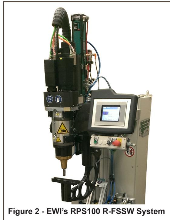
Figure 2 - EWI's RPS100 R-FSSW System
