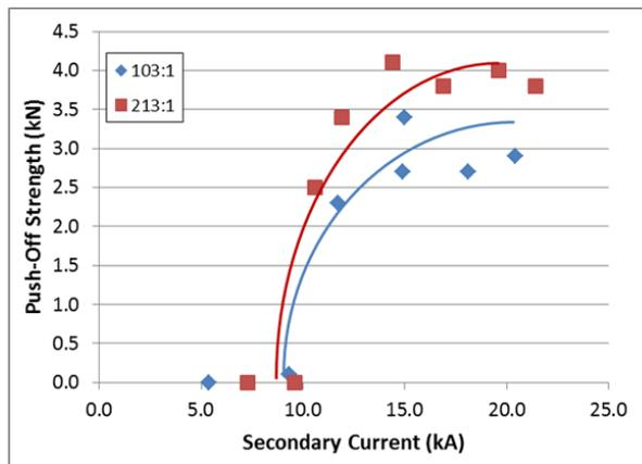
**Figure 11. Process Range Based on Secondary Current for Two Different Transformer Turns-ratios (ratios include 103:1 and 213:1)**
