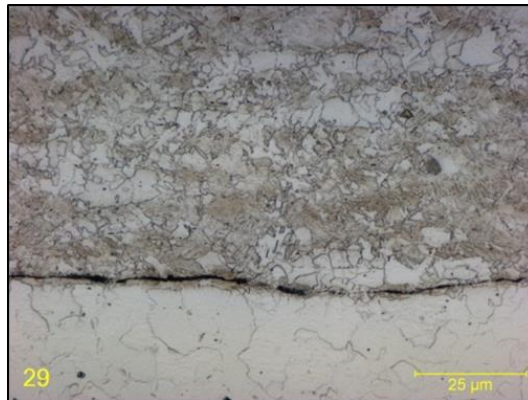
Figure 15. Microstructural Details of the Bondline on a CD Weld Made with a Turns-ratio of 103:1 (note retained ferrite on both sides of the joint)
