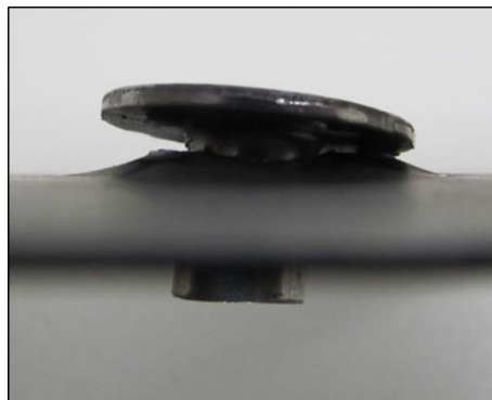
Figure 9. Actual Nut Welded to a 0.8-mm Sheet Steel Following Push-Off Testing
