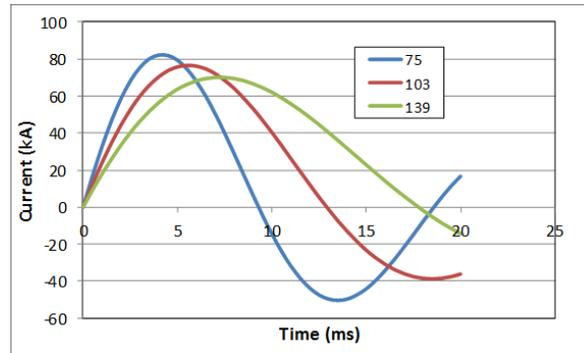
**Figure 4. Influence of Windings Ratio on Current Flow for CD Welding ( $V_c = 1500\text{V}$ ,  $C = 2000 \mu\text{F}$ ,  $R_s = 80 \mu\Omega$ ,  $L_s = 760 \mu\text{H}$ )**
