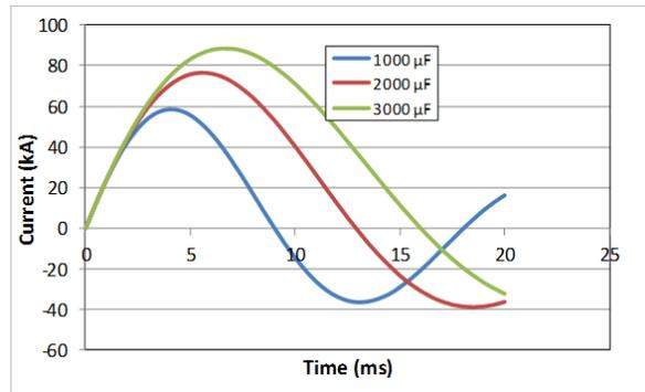
**Figure 3. Influence of System Capacitance on Current Flow for CD welding ( $V_c = 1500\text{V}$ ,  $N = 200:1$ ,  $R_s = 80 \mu\Omega$ ,  $L_s = 760 \mu\text{H}$ )**
