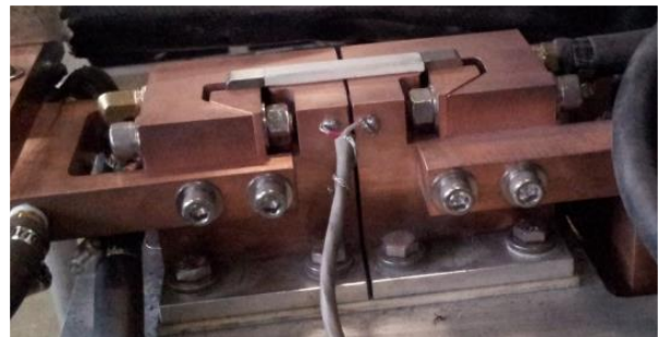
Figure 5. The Coated Mo-TZM Heating Element Positioned by the Tooling in the Pedestal Welding Machine
