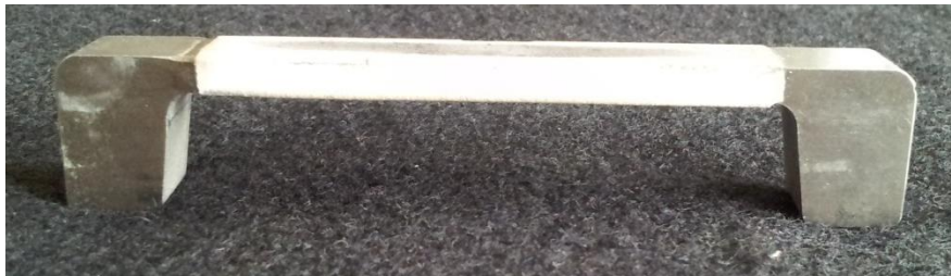
Figure 3. An Example of an Ceramic Coated TZM Heating Element for the Indirect Resistance Heat Treatment Process
