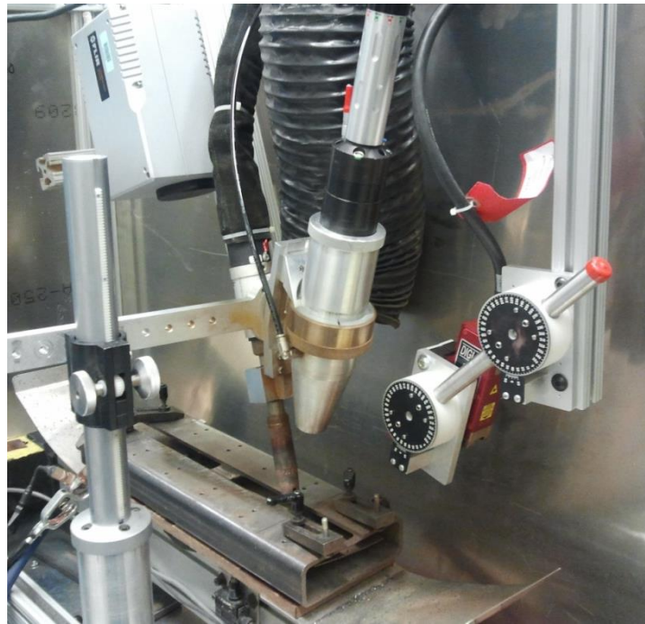
FIGURE 1. Welding system with FLIR camera, GMAW torch, welding laser, and laser profilometer.
