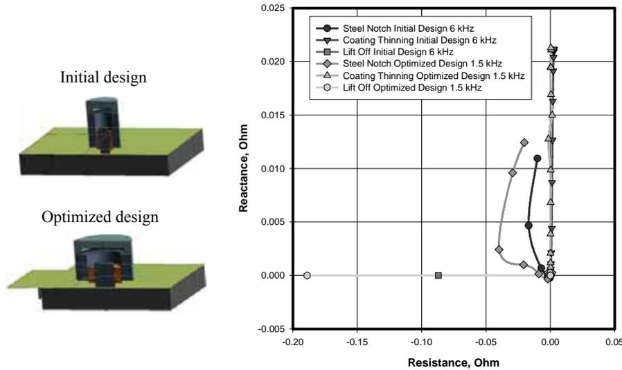
**FIGURE 3.** Solid models and simulated lift off, coating thinning, and notch under coating signals at frequency of 6 kHz and 1.5 kHz for initial and optimized probe geometry with double coil.
