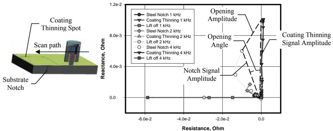
**FIGURE 1.** Solid model (left) and simulated notch and coating thinning signals (right) for pencil probe over steel substrate with aluminum alloy coating at three frequencies.
