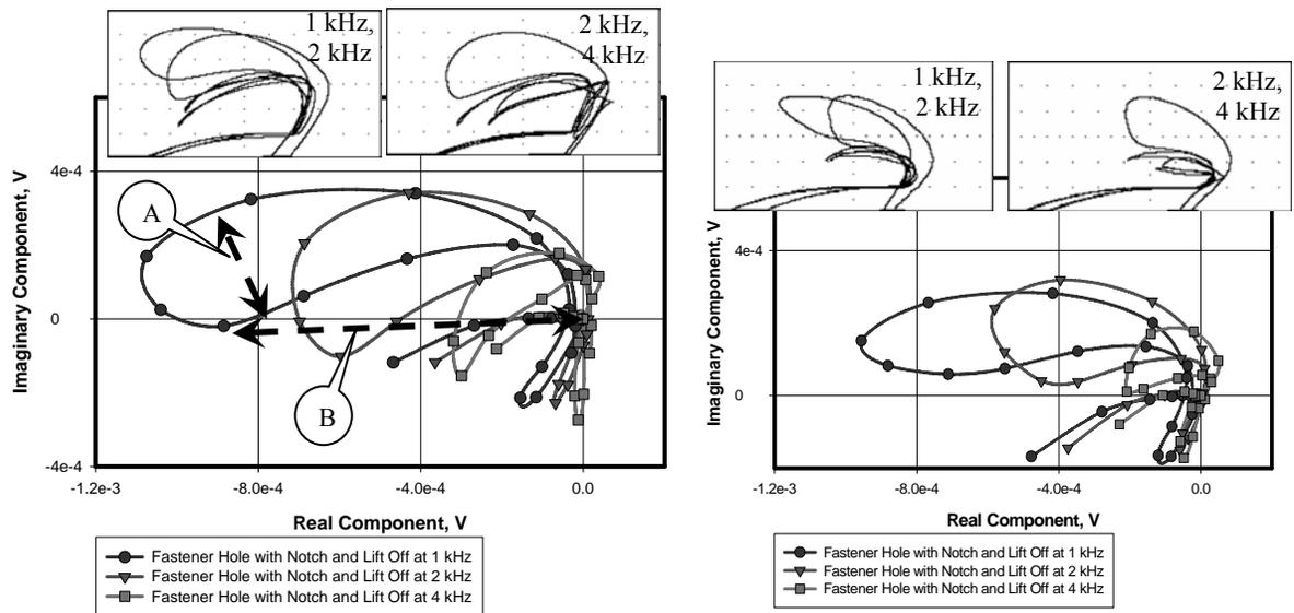
**FIGURE 5.** Simulated and actual fastener holes signals with notch in the third layer obtained with sliding probe at 1, 2 and 4 kHz. Aluminum (left) and titanium (right) alloy fasteners. Conductivity of FHI is assumed “0” (no contact).
