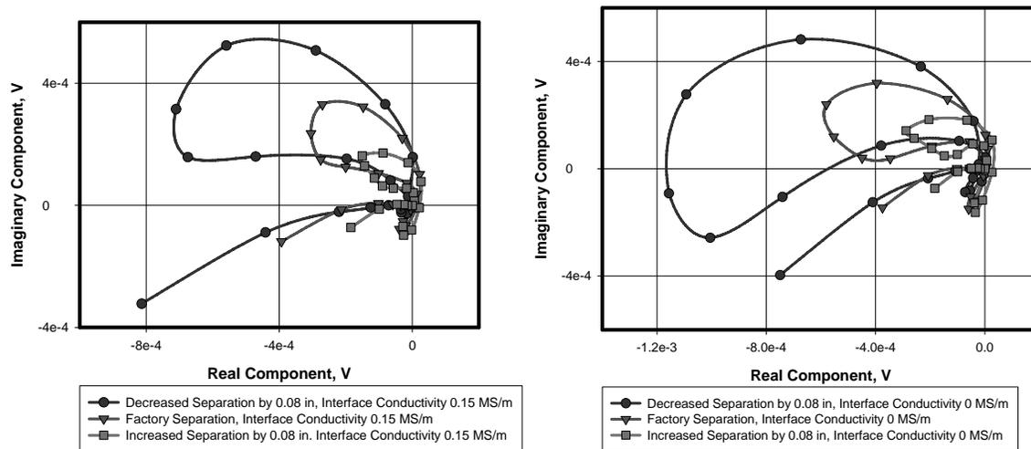
**FIGURE 7.** Simulation of coil separation effect on signals from fastener holes with notch in the third layer and aluminum (left) and titanium (right) fasteners at 2 kHz.
