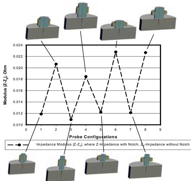
**FIGURE 2.** Simulated effect of probe geometry (core diameter, coil offset, and coil width) on notch sensitivity for probe with ferrite core field concentrator at 6 kHz.
