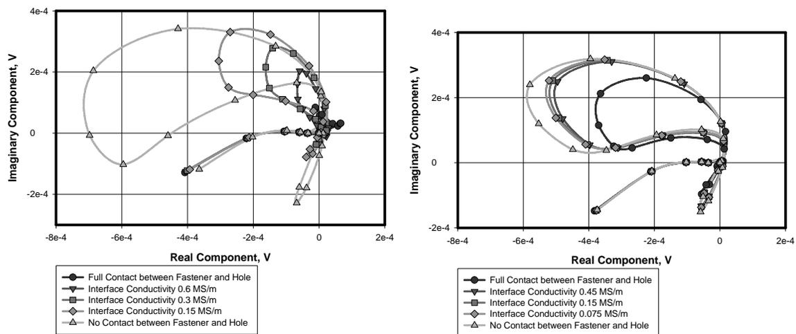
**FIGURE 6.** Simulation of fastener-to-hole interface conductivity effect on signals from fastener holes with notches in the third layer with aluminum (left) and titanium (right) alloy fasteners at 2 kHz.
