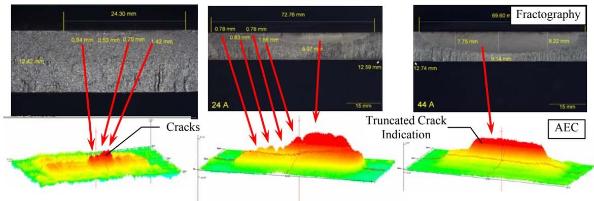
**FIGURE 5.** Fractography (top) and AEC (bottom) indications for the three fractured specimens W41 (left), W24 and W44 (right).
