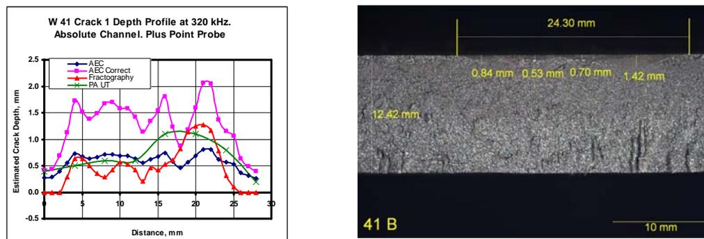
**FIGURE 6.** Comparison of corrected and uncorrected depth measurements for AEC to PA-UT and fractography. (Depth profile – left and fractography for W41 – right.)
