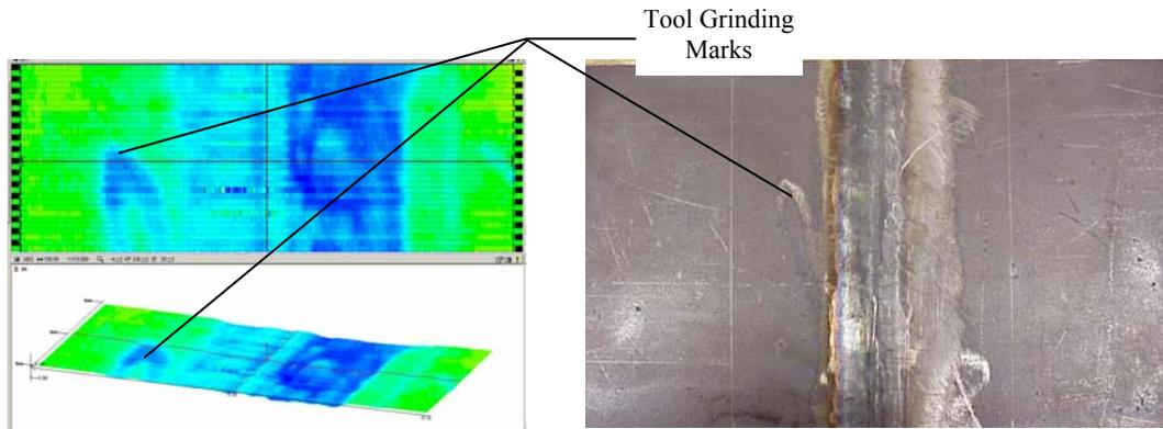
**FIGURE 2.** Typical grinding mark indications on specimen bottom surface.
