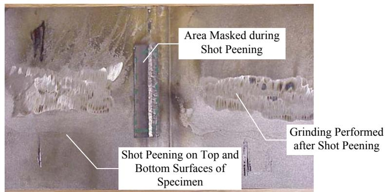
**FIGURE 1.** Specimen with butt weld and three surface areas – shot peened, masked, and ground. The entire bottom surface was shot peened.
