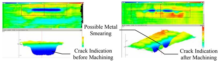
**FIGURE 7.** Comparison of crack indication at 20 kHz on Specimen W44 before (left) and after (right) crown machining acquired with the same probe.
