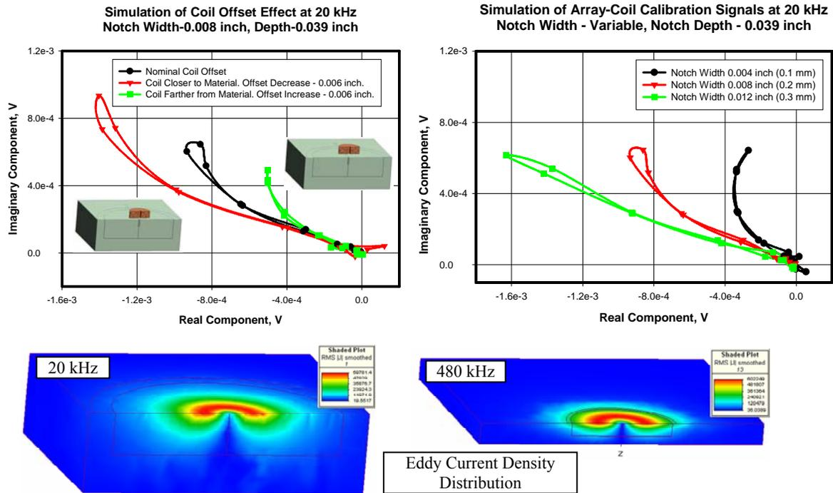
**FIGURE 3.** Modeling the LO and notch width effect (top) and eddy current density distribution (bottom).
