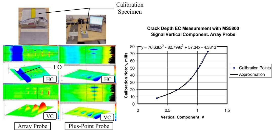
**FIGURE 4.** Calibration for depth sizing with array and single plus-point probe (left) and depth-sizing curve using vertical or imaginary signal component (right). (HC – horizontal signal component, VC- vertical signal component)
