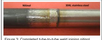
Figure 3: Completed tube-to-tube weld joining nitinol stainless steel
