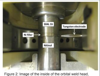
Figure 2: Image of the inside of the orbital weld head, showing the assembled components of the tube-to-tube joint
