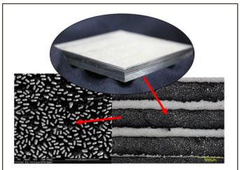
Figure 1: Cross section of a Fabrisonic MMC shown at sequentially higher magnifications
