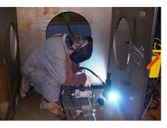
EWI was able to increase the deposition rate and use less filler material while maintaining the required heat input. This allowed a 33% increase in overall productivity while meeting all mechanical property requirements.
