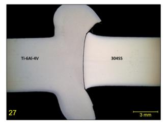
Figure 2: Cross section of an upset weld made between Ti-6Al-4V and 304SS employing a Nb foil at the interface.
