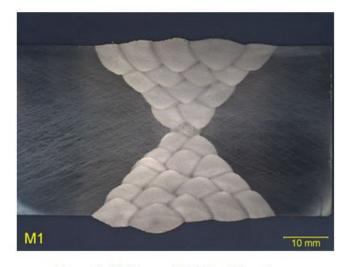
Figure 1: Multi-pass GMAW weld made on 1.5-in thick magnesium
