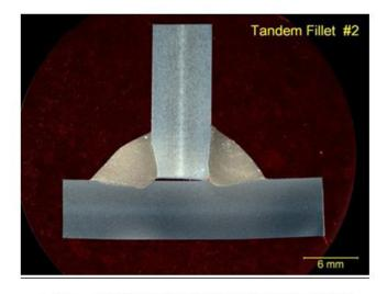
Figure 2: T-GMAW fillet welds made on ¼-in thick 6061 Aluminum at a travel speed of 60-ipm
