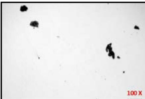
Figure 8: Observed nonmetallic inclusions.
