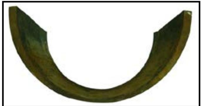
Figure 1: 65% thickness reduction of a 20-in. diameter carbon-steel pip after nine months of operation.
