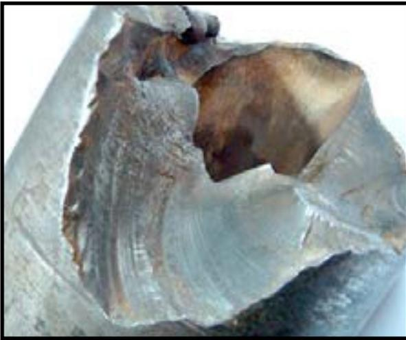
Figure 7: Step pattern fracture zones in the failed upper drive shaft.
