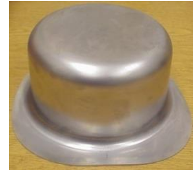
Deep Drawn Sample (6-in. bottom dia. × 3.5-in. depth)
