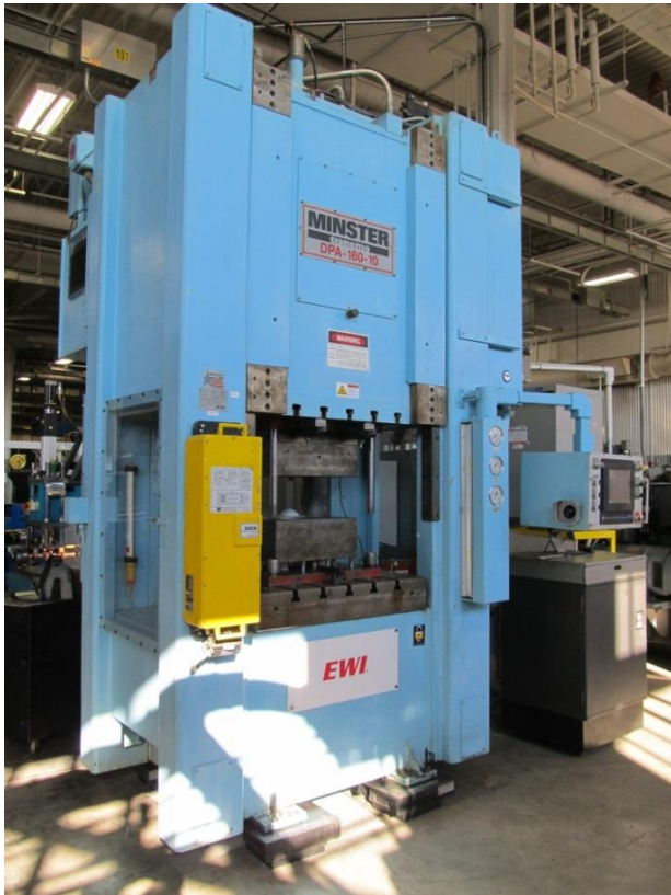
160-ton Minster Tranemo Press (Operating at EWI since Sept. 2012)
