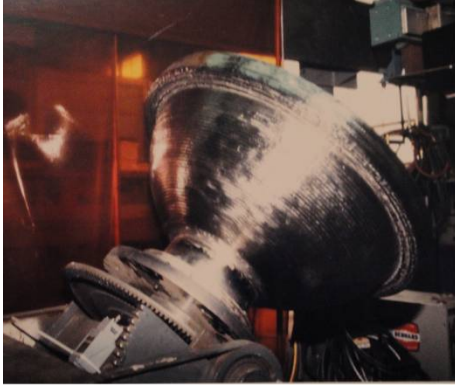
Figure 4. Large component made with robotic arc welding
