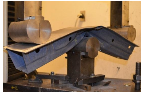
Bend test of PHS part at EWI
