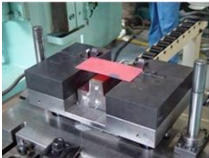
Example hot forming test [Courtesy of POSCO]
