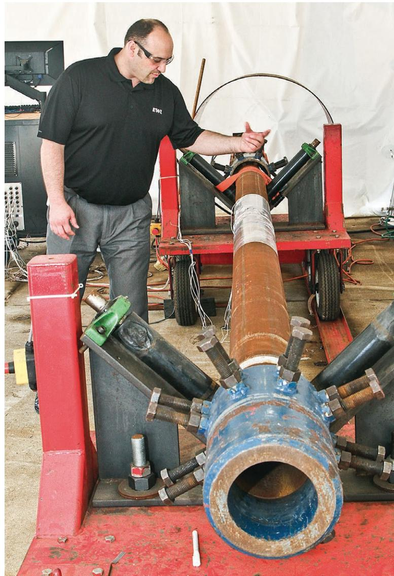
Operations manager Steve Levesque shows off a custom-designed inspection system used in the oil and gas industry to test weld fatigue in pipelines. The device has the capability to evaluate potential stress on a pipeline over its life. In Buffalo, similar test equipment will be built to validate new materials and manufacturing processes.
