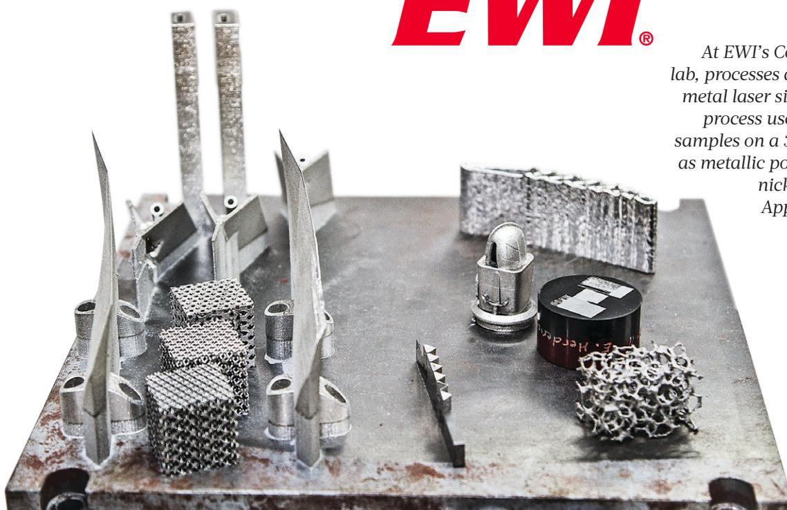
At EWI's Columbus laser sintering lab, processes are developed for direct metal laser sintering, a trademarked process used to create these metal samples on a 3-D printer. They began as metallic powders that can include nickel and titanium alloys. Applications created using this technology are for a variety of industries including aerospace, automotive, heavy manufacturing and consumer products.
