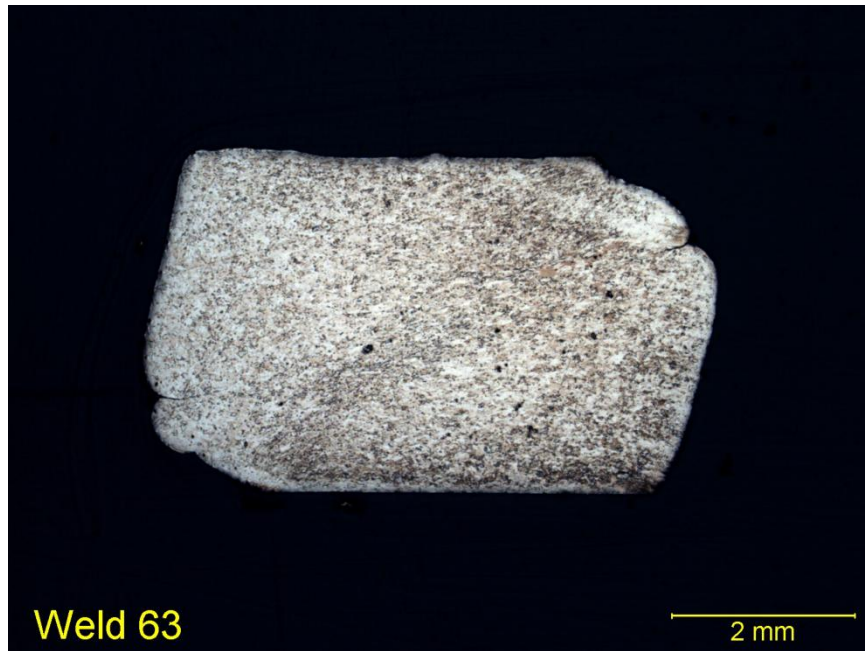
Figure 15. Micrograph of Weld 63 Showing bond and Microstructure of Cross-Wire Joint using Best-Practice Welding Parameters (The section was cut transverse to the wire cross direction.)
