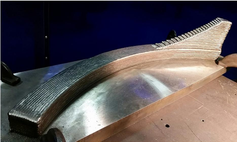
Demonstration part built by EWI to show typical appearance and process control achieved using arc-directed energy deposition (DED) for large parts.
