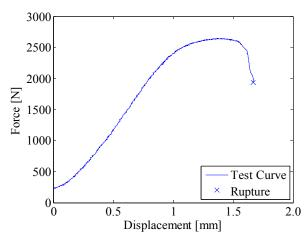
Fig. 9. UAM 1-2 sample force versus displacement curve showing significant plastic yielding, indicating ductile failure of the sample.
