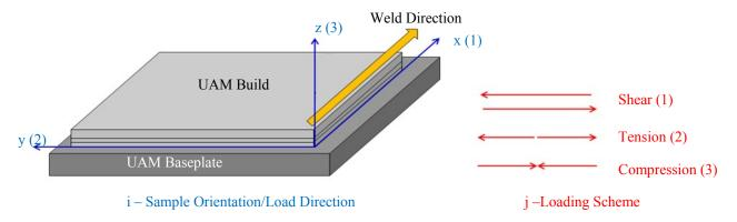
Fig. 5. Indicial notation diagram for UAM mechanical testing samples.
