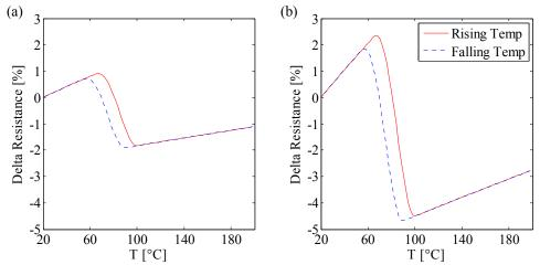
Fig. 12. Resistance model results describing the composite change in resistance versus temperature.
