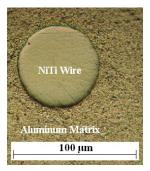
Fig. 4. Micrograph of 75 μm diameter shape memory Ni-Ti wire fully embedded in Al 3003-H18 UAM matrix utilizing only plastic flow of the matrix material.
