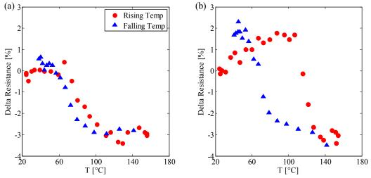
Fig. 10. Experimental Ni-Ti resistance response showing the change in electrical resistance versus temperature.
