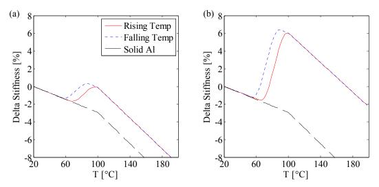
Fig. 13. Ni-Ti composite stiffness versus temperature. (a) 4.5% Ni-Ti area ratio composite. The model indicates there is insufficient NiTi to offset the softening of the matrix with increasing temperature. (b) 13.4% Ni-Ti area ratio composite. The model indicates an increase in composite stiffness with temperature up to approximately 180°C. Both models show an increased stiffness over solid aluminum in the same geometry after the M-A transition.
