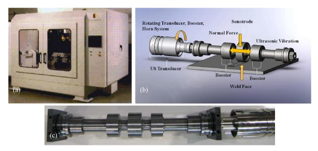
Fig. 2. (a) UAM 'Beta' machine used to manufacture strength testing samples. (Photograph courtesy of Solidica, Inc.) (b) In the UAM process, successive layers of metal tape are bonding together for creating metallic composites with seamlessly embedded materials and features. (c) Rotating transducer, booster and horn system used in UAM.
