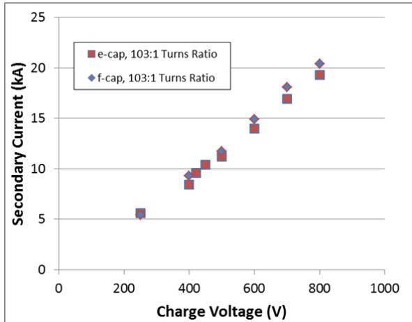
**Figure 9. Relationship between Current and Voltage for both E- and Film-Caps Using a 103:1 Transformer Turns-Ratio**
