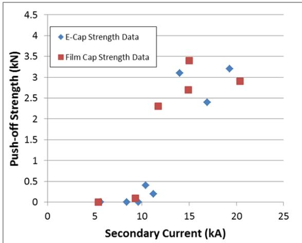
**Figure 11. Current Range Results Based on Weld Strength for both E- and Film-Caps Using a 103:1 Transformer Turns-Ratio**
