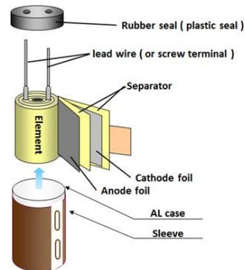
**Figure 4 – Packaging of an Electrolytic Capacitor** (note continuous foils and separator)
