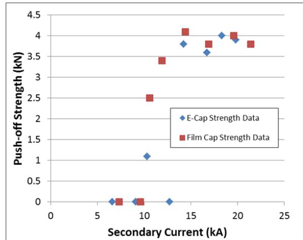
**Figure 12. Current Range Results Based on Weld Strength for both E- and Film-Caps Using a 213:1 Transformer Turns-Ratio**
