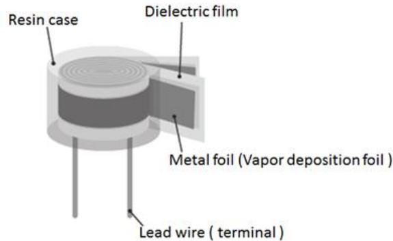
**Figure 2. Packing of a Film-type Capacitor into a Cylindrical Configuration** (package can be wound for either cylindrical or prismatic designs)
