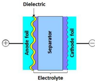
**Figure 3. Schematic Representation of the Foil-Separator Layout in an Electrolytic Capacitor**
