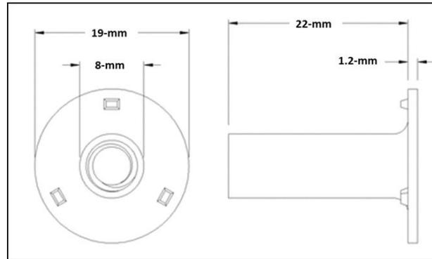
**Figure 8. Design of the Weld Nut Used in This Study** (weld nuts were of mid steel, with three projections nominally 2.5 mm in diameter and 0.95-mm tall)
