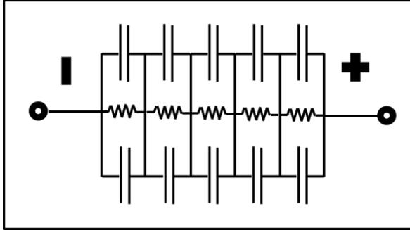
**Figure 5. Design of the Capacitor Array used in this Study** (included five sets of two capacitors in parallel each placed in series; note the balance resistors between each parallel capacitor set)
