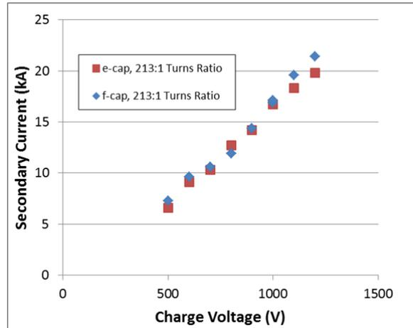
**Figure 10. Relationship between Current and Voltage for both E- and Film-Caps Using a 213:1 Transformer Turns-Ratio**
