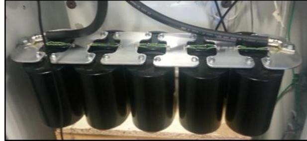
**Figure 6. Actual Array of Capacitors Used in This Study** (note the large aluminum shunts coordinating the capacitors in the series and parallel configuration, and the balancing resistors)
