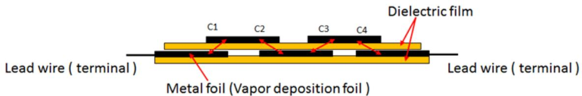
**Figure 1. Conceptual Layout of a Film Type Capacitor** (includes alternating charge plates separated by a dielectric film)
