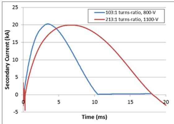
**Figure 7. Secondary Current Response for Two Different Windings Ratios using a Film-cap in the Power Supply<sup>(1)</sup>** (charge voltage is adjusted to achieve similar peak currents)
