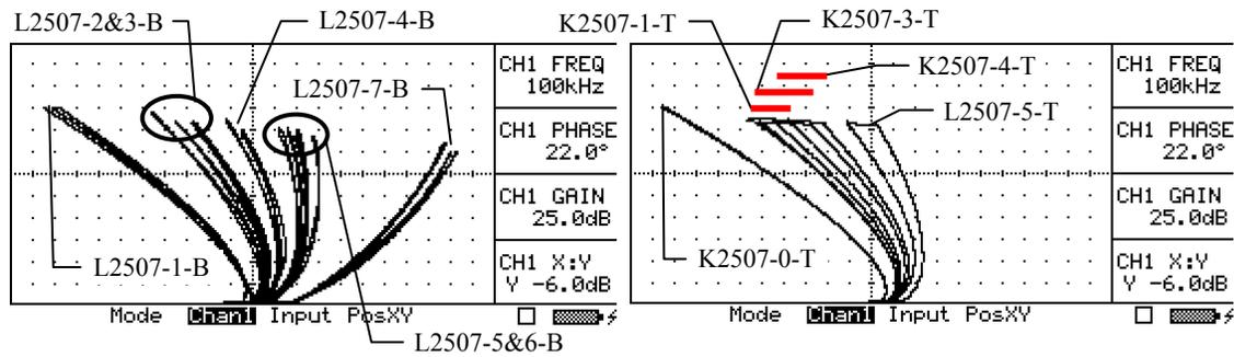
**FIGURE 2.** Typical conventional eddy current sorting at 100 kHz.
