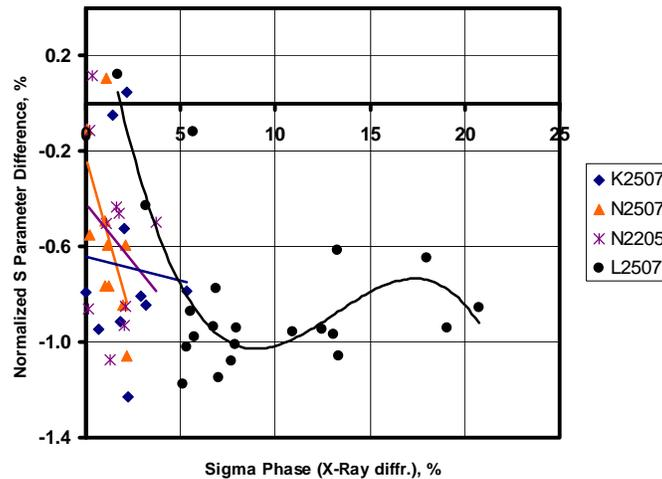
**FIGURE 7.** Normalized S parameter (IPA-V) difference versus SP (measured with X-Ray diffraction) for K2507, N2507, N2205, and L2507.
