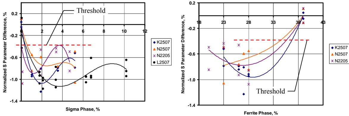
**FIGURE 5.** Normalized S parameter (IPA-V) difference versus SP and FP for K2507, N2507, N2205, and L2507.
