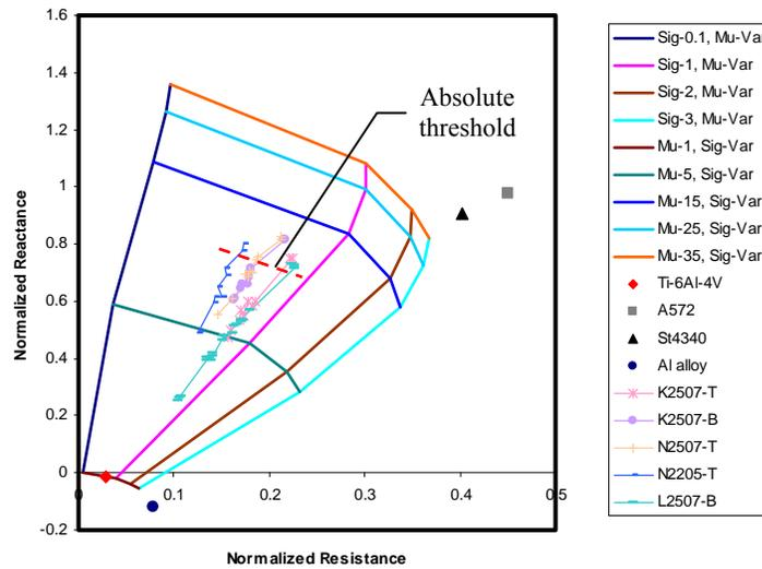
**FIGURE 3.** Simulated and measured impedance loci at 25 kHz.
