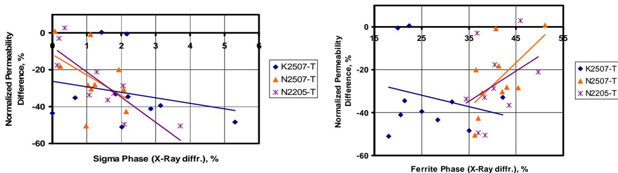
**FIGURE 6.** Normalized magnetic permeability difference versus SP (left) and FP (right) for K2507-T, N2507-T, and N2205-T at 25 kHz (both phases measured with X-Ray diffraction).
