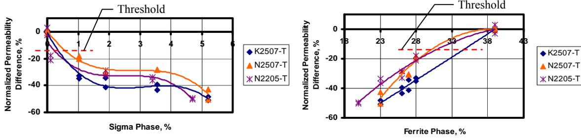
**FIGURE 4.** Normalized magnetic permeability difference versus SP and FP for K2507-T, N2507-T, and N2205-T at 25 kHz.
