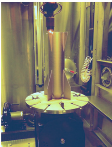
Figure 1: Demonstration part being built using the RPMI 557 L-DED system
