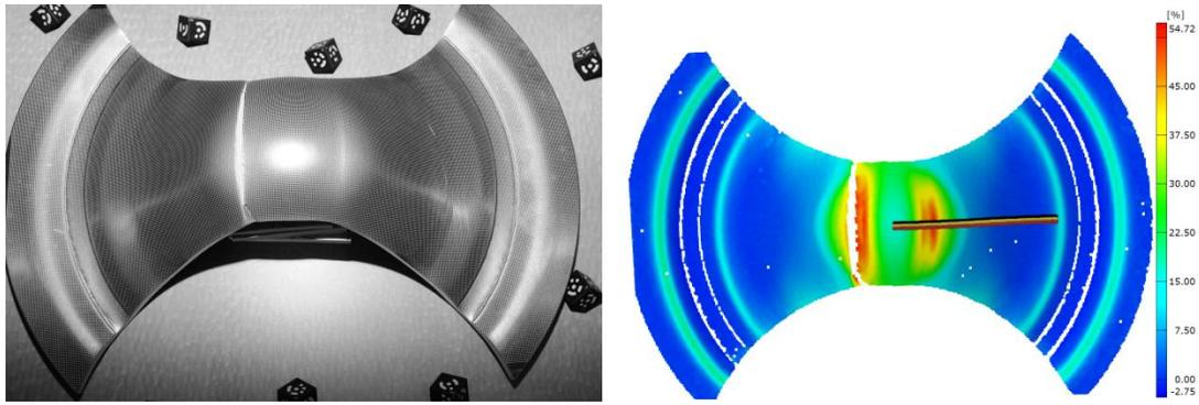
Figure 3: A tested sample for FLD analysis (left) and the measured stain distribution using the ARGUS system (right)
