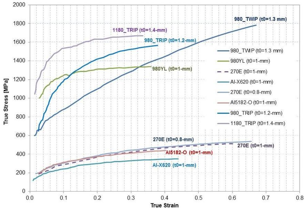
Figure 2: The stress-strain data obtained from the VPB test
