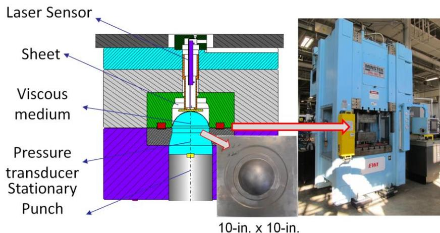
Figure 1: VPB testing for sheet material at EWI's 160-Ton hydraulic press
