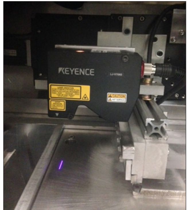
Figure 3. A commercial laser vision system will need to be modified or developed to be commercially viable for real-time surface inspection in a laser powder bed AM process.
