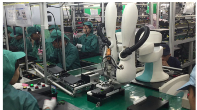
Figure 2: Kawasaki Robotics duAro cobot working on an electronics assembly line (courtesy of Kawasaki Robotics)
