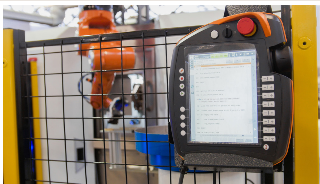
Figure 1: A robotic material-handling system guarded by fencing
