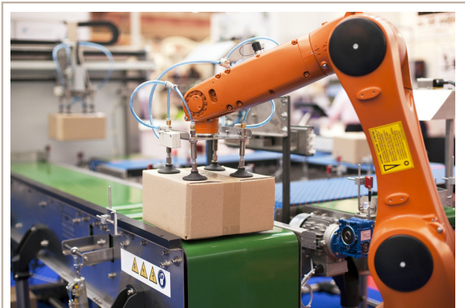
Figure 3: Robotic arm performing a packing operation
