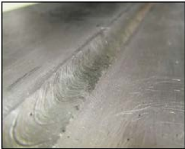
Figure 4: 6061 lap joint welded at 60 ipm using Tandem GMAW.
