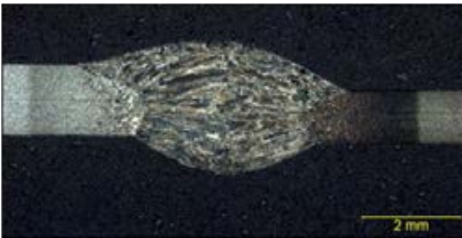
Figure 1: Application of high-speed tandem GMAW to tailor-welded blanks.
