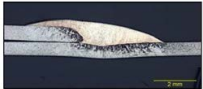
Figure 5: Galvanealed sheet metal joining using silicon bronze electrodes.
