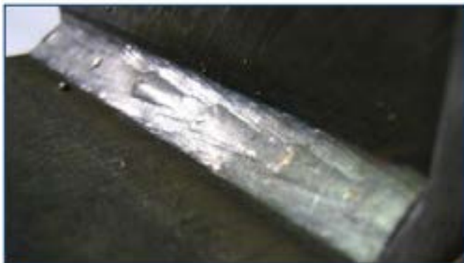
Figure 2: 3/16-in fillet weld made at 80 ipm.
