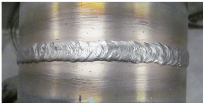
Figure 5: Semi-automatic butt-joint weld produced at Vigor Industrial in the 1G-R position
