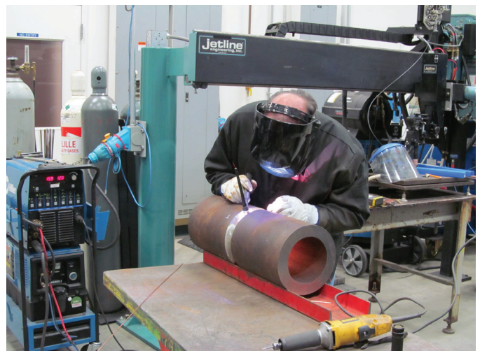
Figure 1. Inserting the tack welds at the root.
