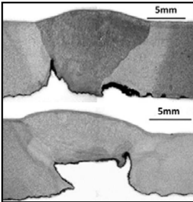
Figure 5: Corrosion of gas pipeline welds due to welding imperfections.
