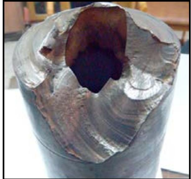
Figure 6: General view of the failed drive shaft after approximately 245,000 revolutions.
