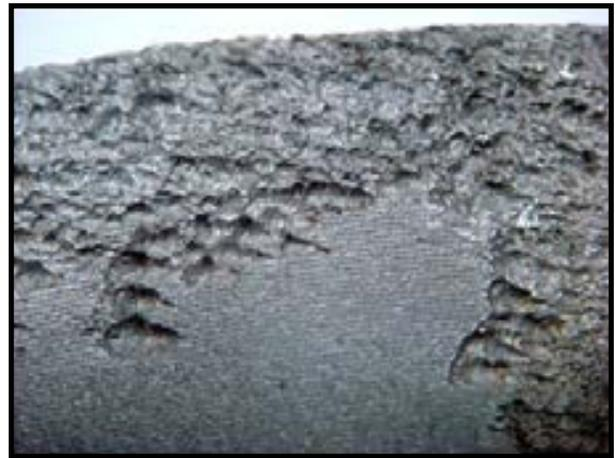
Figure 3: Evidence of the direction of flow on the eroded impeller surface.
