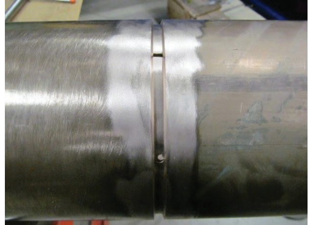
Figure 1: Butt joint with backing ring.
