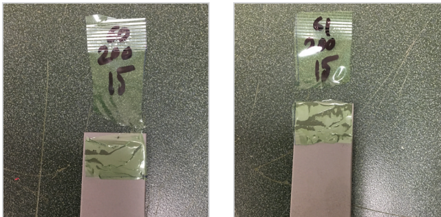
Figure 9. Failure mode for bonding of thinner PA to blasted steel, and one of the bonds to the hydroxyapatite coating
