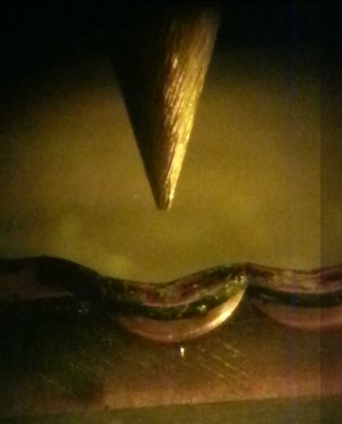
Magnified photo of edge welds on copper
