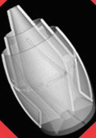
CT scan of a jet propulsion component
