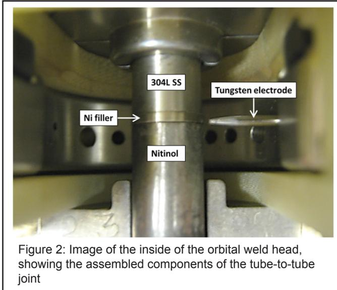
Figure 1 shows the unassembled components of the weld joint. Figure 2 provides an image of the inside of the welding head, with the tubes and insert assembled and positioned relative to the tungsten electrode.
