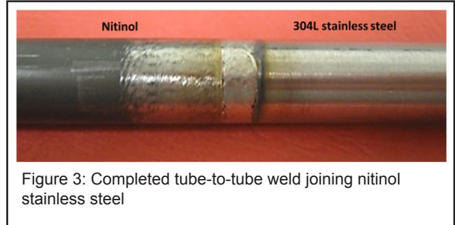
Six identical tube assemblies were then welded and tested by EWI's research partner in their laboratory. Torque strength was measured through several thousand thermal cycles, and repeatability of position-at-temperature was excellent, demonstrating the feasibility of this manufacturing approach.
