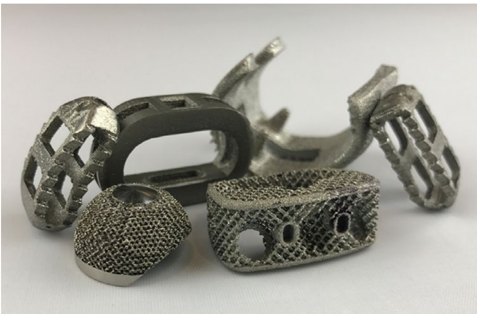
Figure 1: Orthopedic devices built using EB-PBF New Design Capabilities
