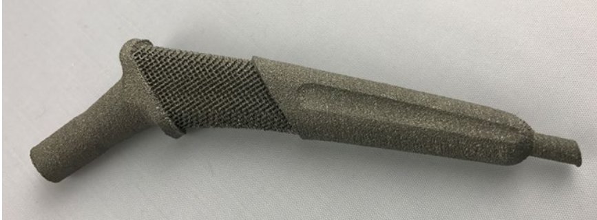
Figure 3: Ti-6Al-4V femoral stem manufactured using EB-PBF (Photo provided courtesy of Arcam AB)
