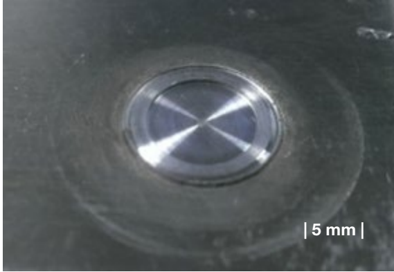
Figure 4: Top surface of an aluminum refill friction stir spot weld
