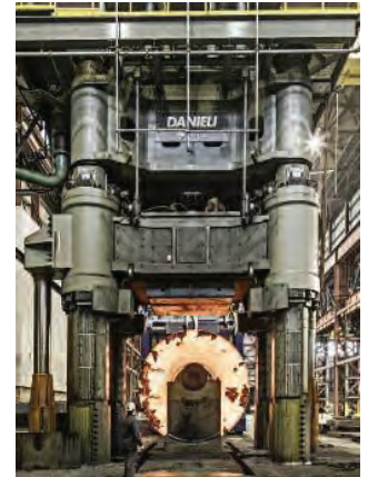
4.9 m diam. X 1.2 m thick at ~91,000 kg forging. Image sup by North American Forgemasters/Scot Forge
