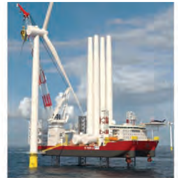
Shipbuilder: Keppel Location: Texas Name: Charybdis Wind Turbine Installation Vessel 144m (462 ft) $500M 2024 launch
