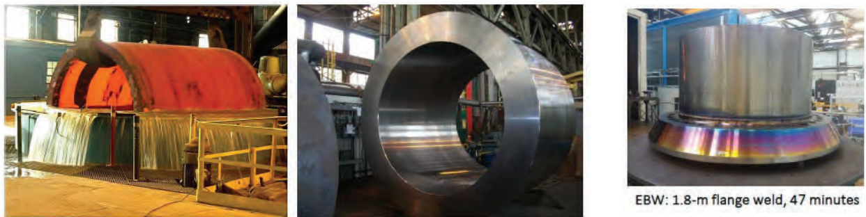
Examples of forging during heat treatment and after machining. Image supplied by Lehigh Heavy Forge Corp.
