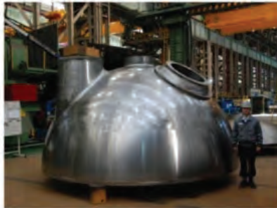
Steam generator channel head
