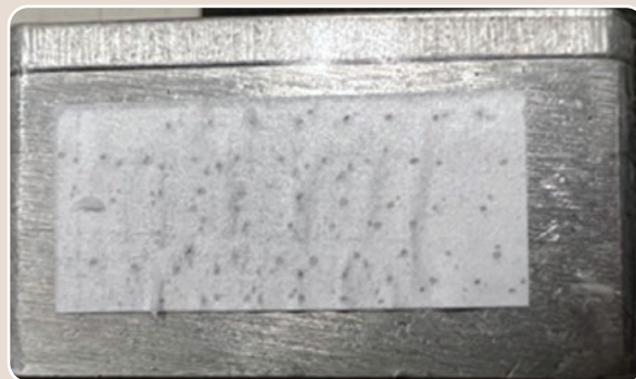
Figure 17b: LeakSight tape applied
