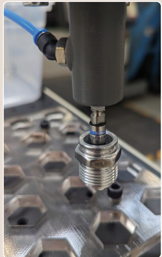
Figure 14: Fixturing and inner diameter grip for robotic deburring
