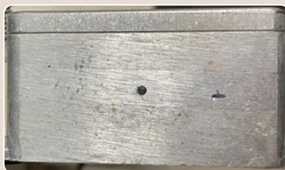
Figure 17a: Box with 300 µm hole
